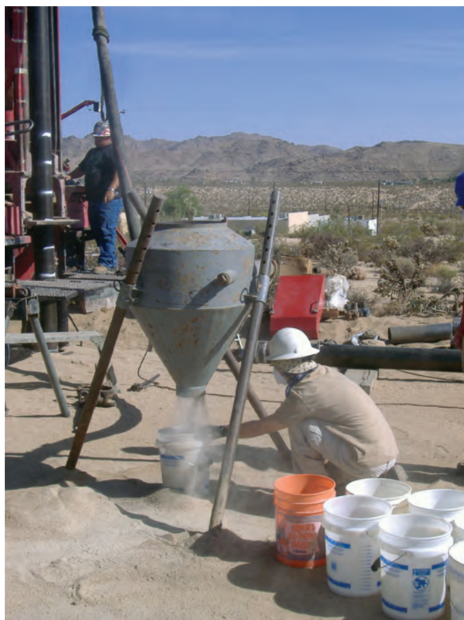
Figure 3. Collection of ODEX drilling cuttings from “cyclone” discharge, in Joshua Tree, San Bernardino County, California, May 2007
