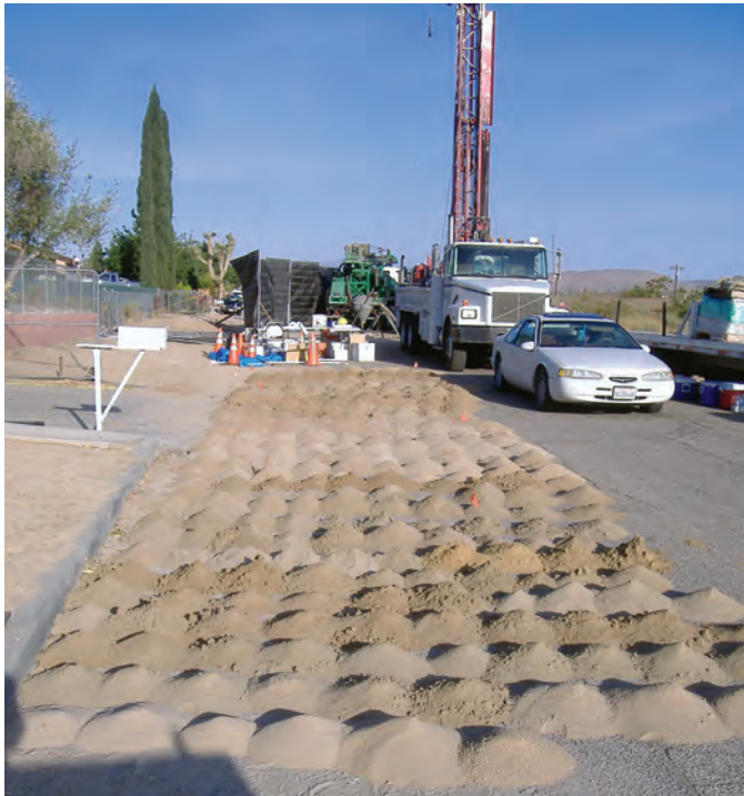
Figure 5. ODEX cuttings arranged so that major lithologic changes could be identified, 1N/6E-35A1 (JTUZ-1), Joshua Tree, San Bernardino County, California, May 2007
