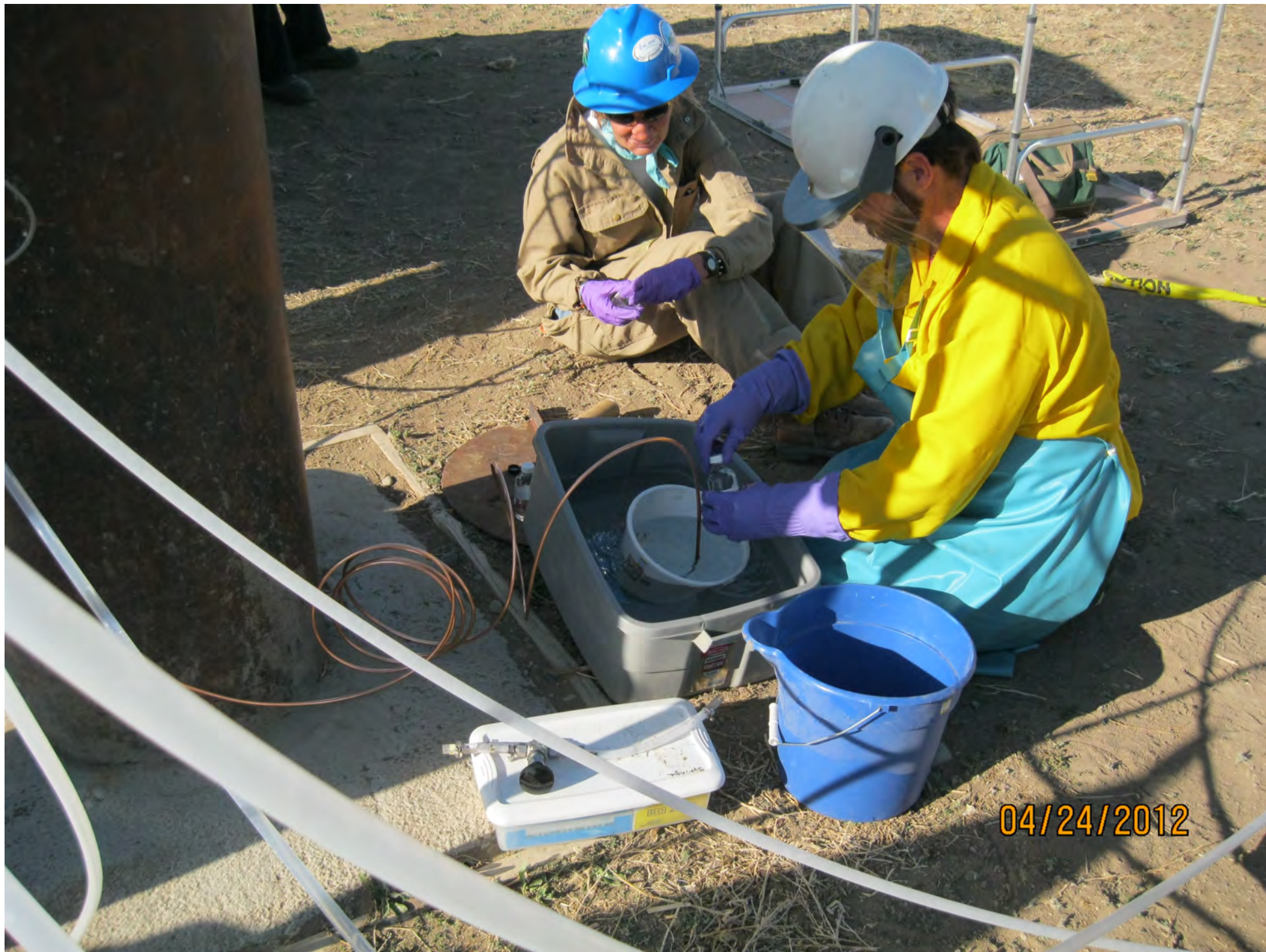
Figure 3.13. Collection of dissolved gas samples beside well head. Photograph by Tom Kropatsch, Wyoming Oil and Gas Conservation Commission, April 24, 2012.
