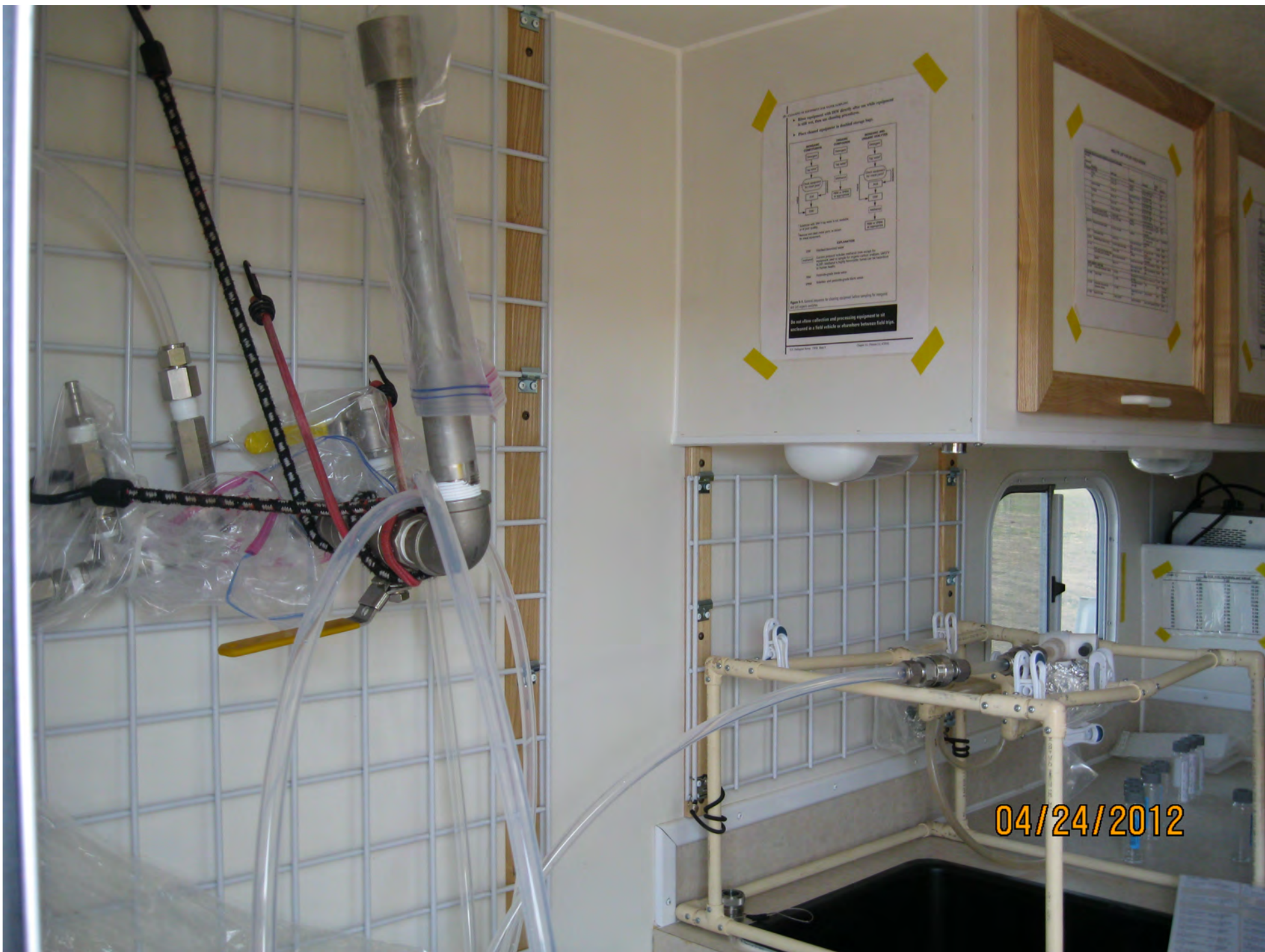
Figure 3.4. U.S. Geological Survey blank sample collection setup, including a piece of flow manifold and sampling lines used during sample collection, Photo by Tom Kropatsch, WOGCC.
