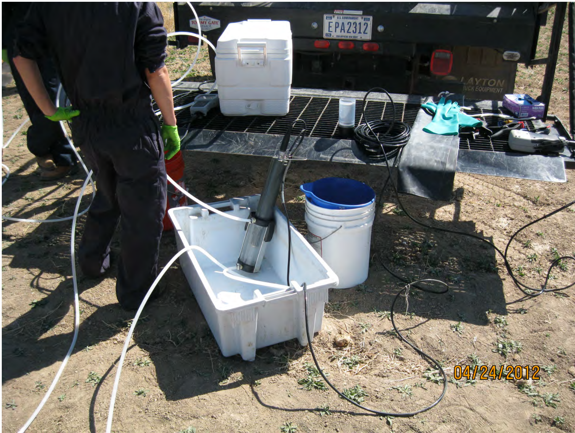
Figure 3.6. Water-quality instrument with flow cell measuring water temperature, pH, specific conductivity, dissolved oxygen and oxidation reduction potential, Photo by Tom Kropatsch, Wyoming Oil and Gas Conservation Commission.
