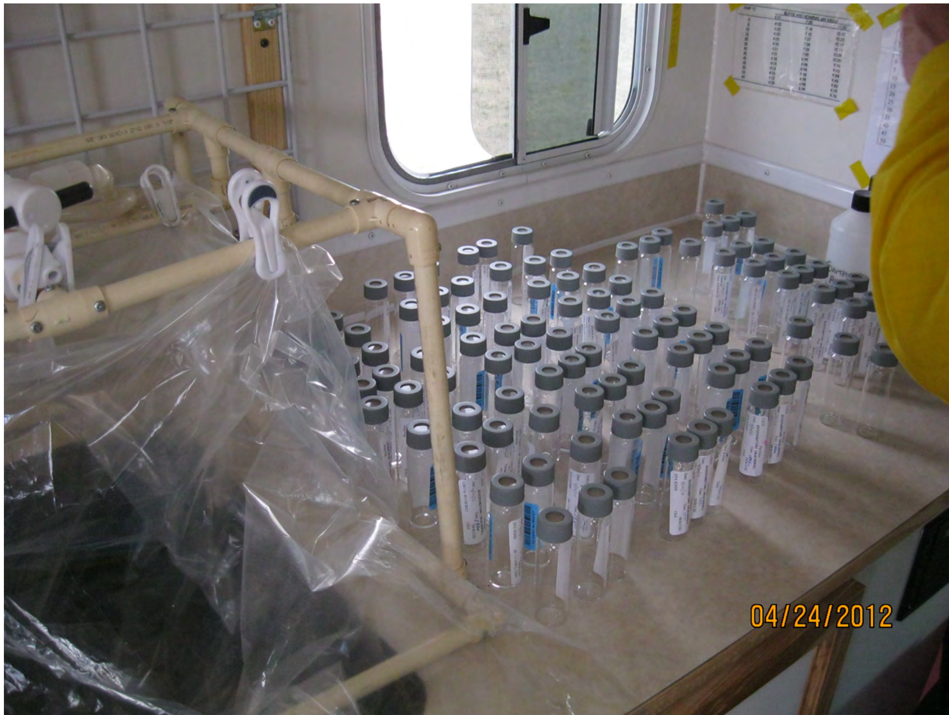
Figure 3.8. VOC vials being labeled in preparation for sampling Monitoring Well MW01. Photograph by Tom Kropatsch, Wyoming Oil and Gas Commission, April 24, 2012.
