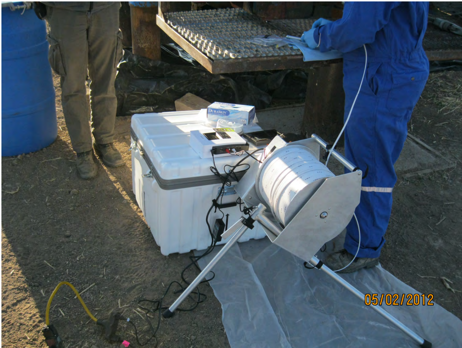
Figure 6.5. Downhole camera setup. Photograph by Tom Kropatsch, Wyoming Oil and Gas Conservation Commission, May 2, 2012.
