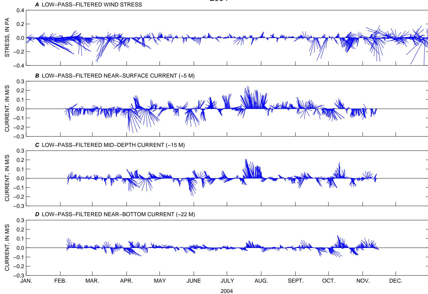
Low-Pass-Filtered Wind Stress at NOAA Buoy 44013 and Selected ADCP Observations at LT-A
