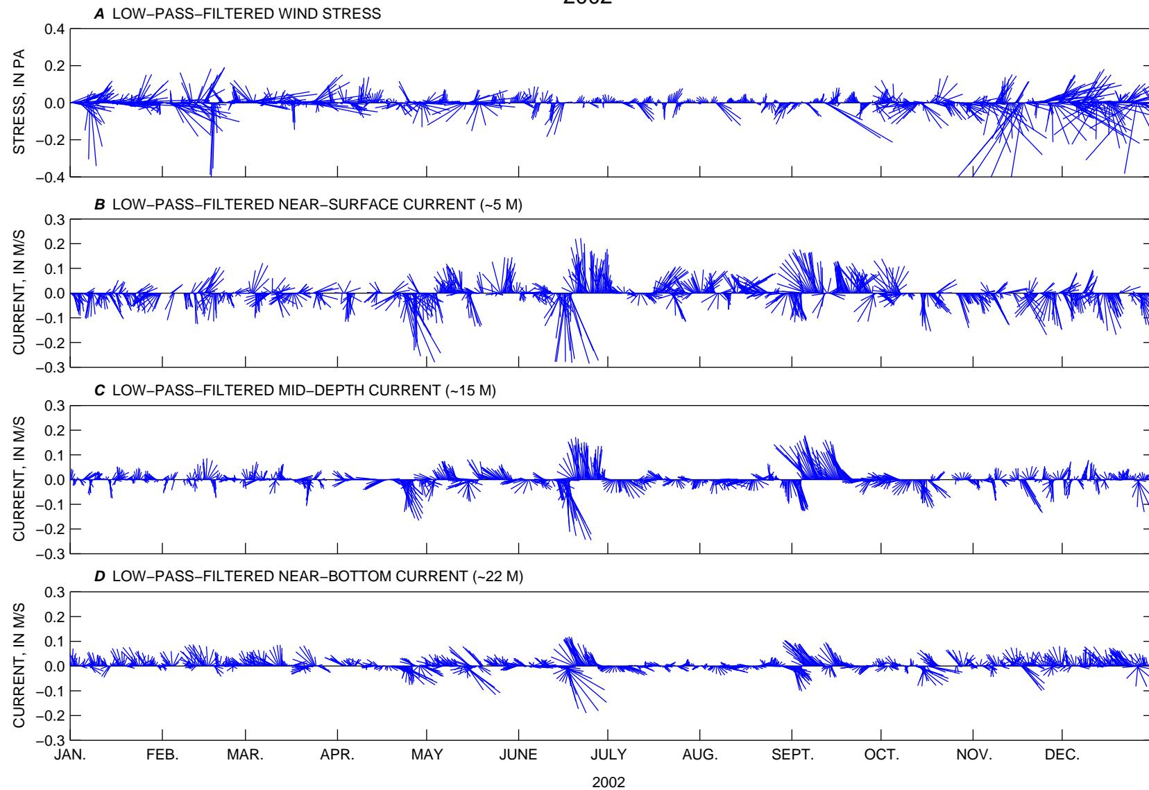
Low-Pass-Filtered Wind Stress at NOAA Buoy 44013 and Selected ADCP Observations at LT-A
