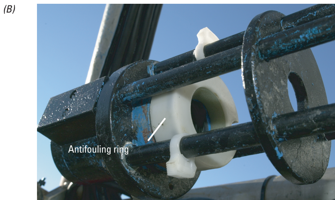
Figure 23. (A) A Sea-Tech 25-centimeter folded-path transmissometer mounted horizontally on the large tripod frame (see fig. 4A) and (B) a Delrin(TM) anti-fouling ring (white ring) mounted around the transmissometer window. Photographs by Dann Blackwood, U.S. Geological Survey.
