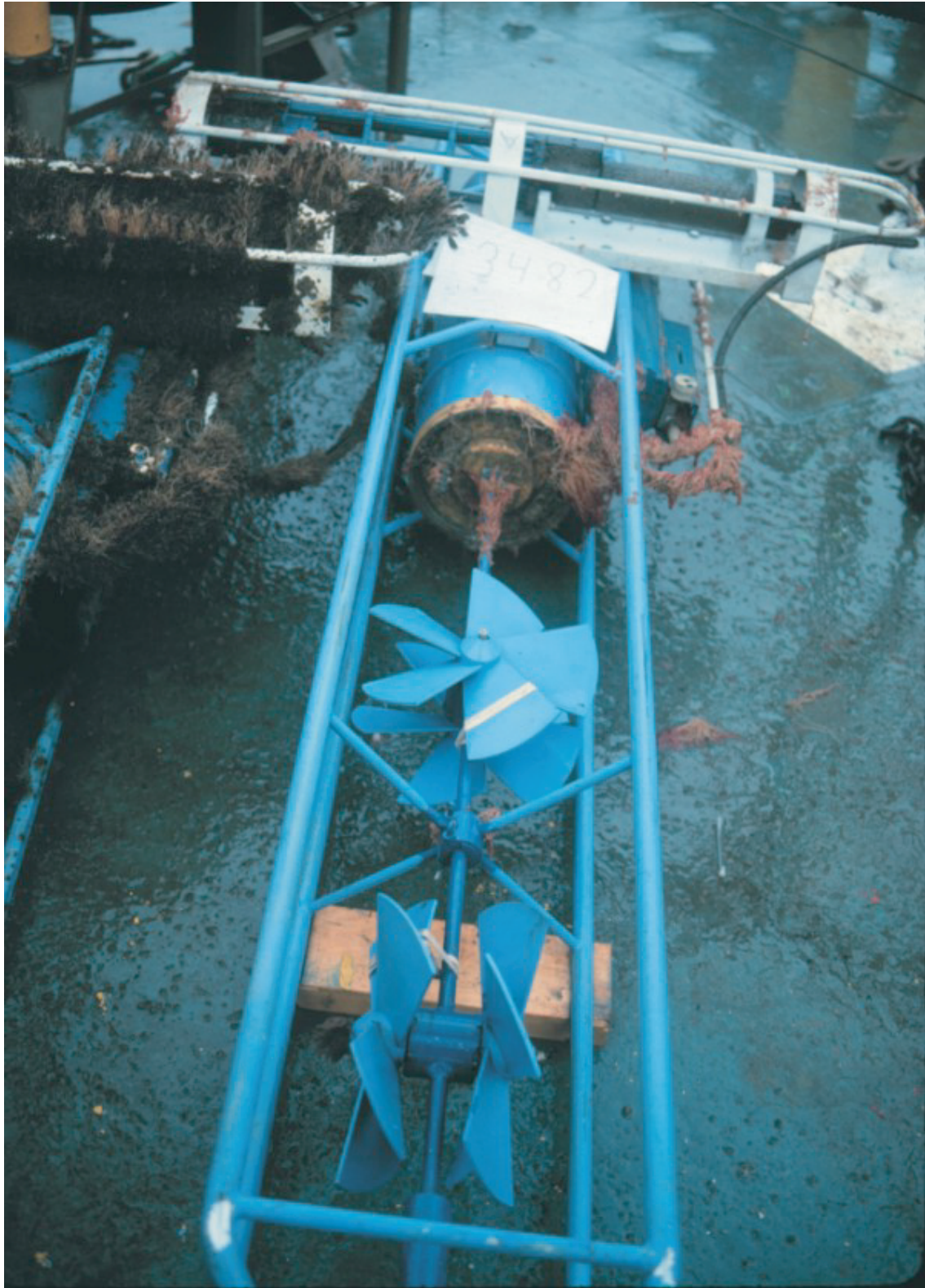
Figure 28A. A Vector-Measuring Current Meter (VMCM) deployed on mooring 348 at about 22 meters (10 meters above bottom) from July to October 1990. The blue and white color is antifouling paint. Note the growth on the unpainted lower end cap of the instrument housing, and slight growth on the rotor hub. Photograph by Bradford Butman, U.S. Geological Survey
