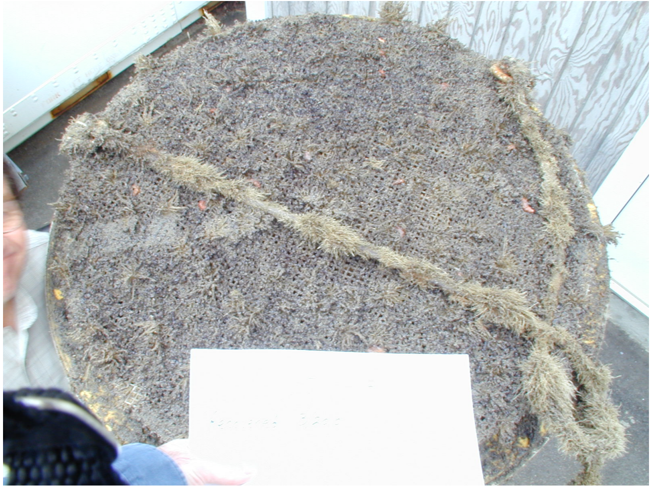
Figure 31. The top of a time-series sediment trap with exceptional bio-fouling (estimated 95-percent coverage) after a summer deployment (May 2000 to September 2000) at site LT-B. The line across the baffle is a section of the three-part nylon rope mooring bridle. A nylon screen (1 centimeter grid) and a plastic honeycomb baffle are placed at the open end of the trap funnel in order to reduce turbulence and to prevent large animals from entering the trap. The trap opening is 0.8 meters in diameter.
