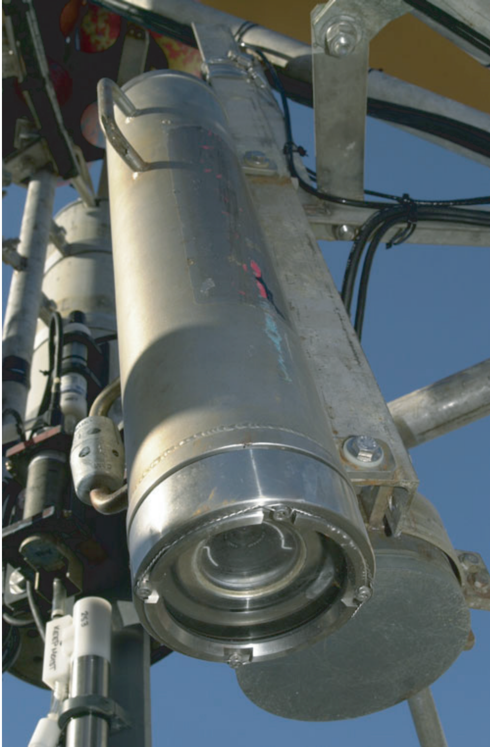
Figure 18. Benthos 35-millimeter underwater camera mounted on tripod frame (shown in fig. 4A). Photograph by Dann Blackwood, U.S. Geological Survey.
