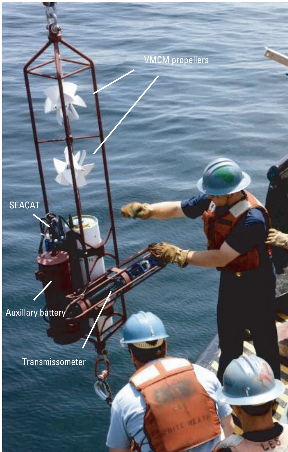
Figure 20. Vector Measuring Current Meter (VMCM) being deployed at site LT-A. The VMCM uses two bidirectional propellers mounted at right angles to measure current. A SEACAT data logger, which measures temperature, conductivity, and light transmission, is bolted to the VMCM frame. Beginning in February 1998, the SEACAT was no longer attached to the VMCM and was deployed in a separate frame (see fig. 21). Photograph by Dann Blackwood, U.S. Geological Survey.
