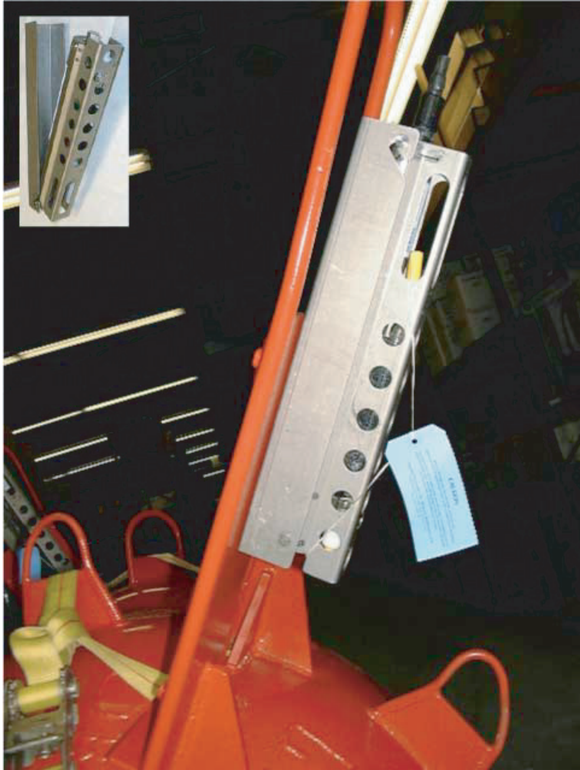
Figure 22. A MicroCAT mounted on the top of a 41-inch steel float. This mounting was used at site LT-A to measure temperature and salinity within about 5 meters of the sea surface. The inset shows a close-up of the MicroCAT installed in a protective bracket. Photograph by Dann Blackwood, U.S. Geological Survey.
