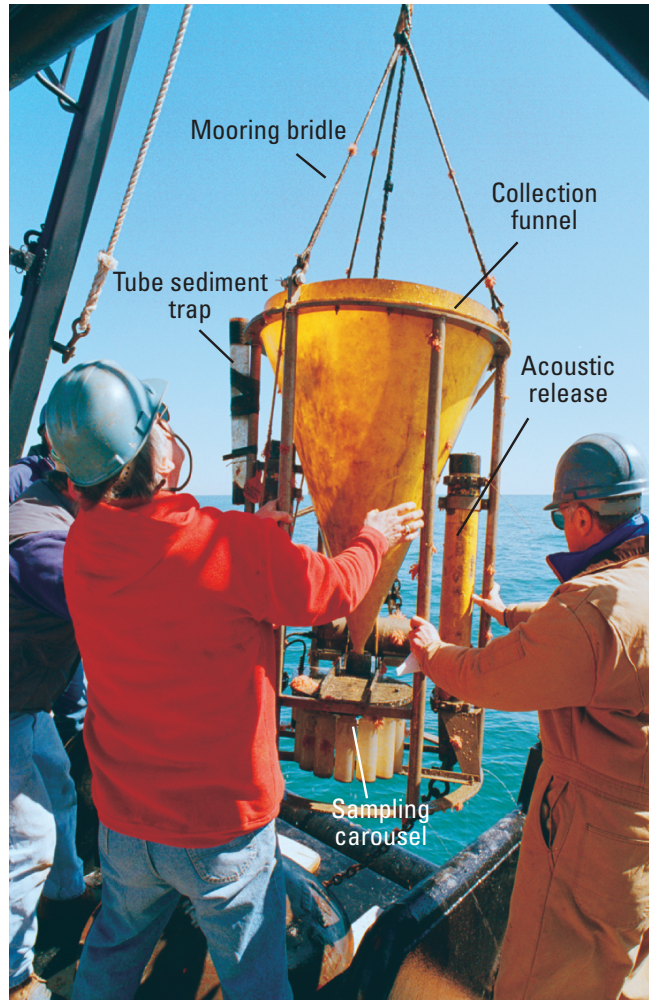
Figure 24. Time-series sediment trap deployed at sites LT-A and LT-B. The yellow funnel (0.8-meter diameter) directs suspended material into one of 13 plastic jars (500-milliter capacity), which are sequentially moved under the funnel for a 9-day interval during a typical 4-month deployment. Photograph by Dann Blackwood, U.S. Geological Survey.
