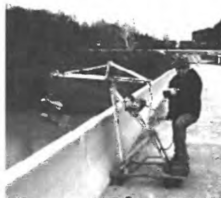
Figure 3. Crane, current meter, and weight used for measuring the discharge of a river from a bridge.
