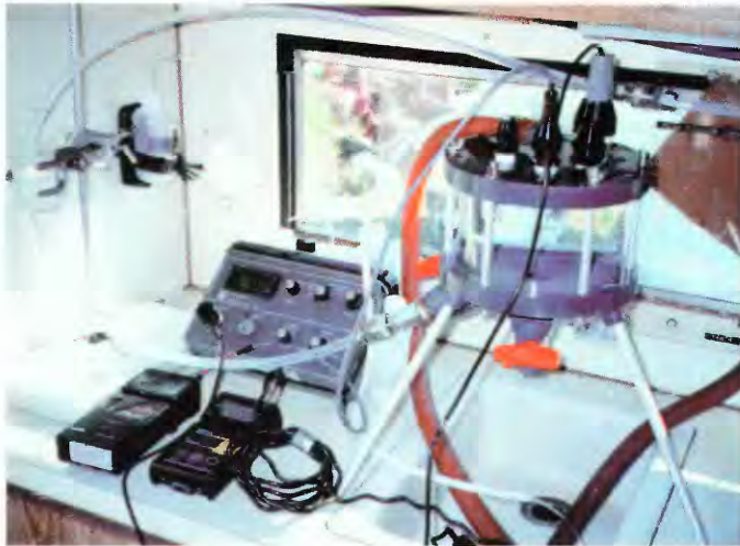
Figure 7. Interior view of mobile laboratory showing equipment used to measure pH, water temperature, specific conductance, and dissolved oxygen.
