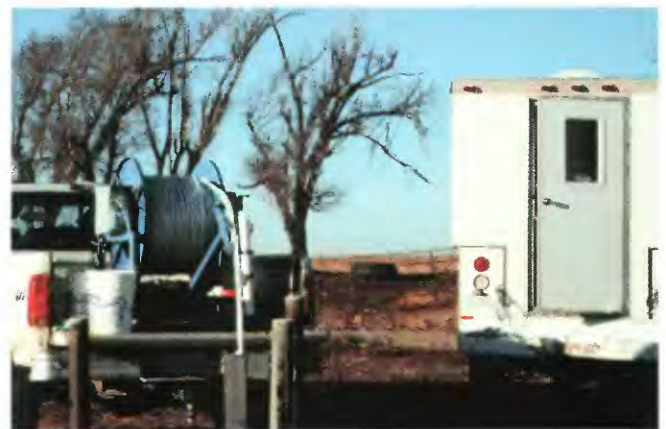
Figure 6. Monitoring wells were pumped using a stainless steel submersible pump mounted in the back of a pickup truck (vehicle on left). Samples were processed inside a mobile laboratory (vehicle on right).
