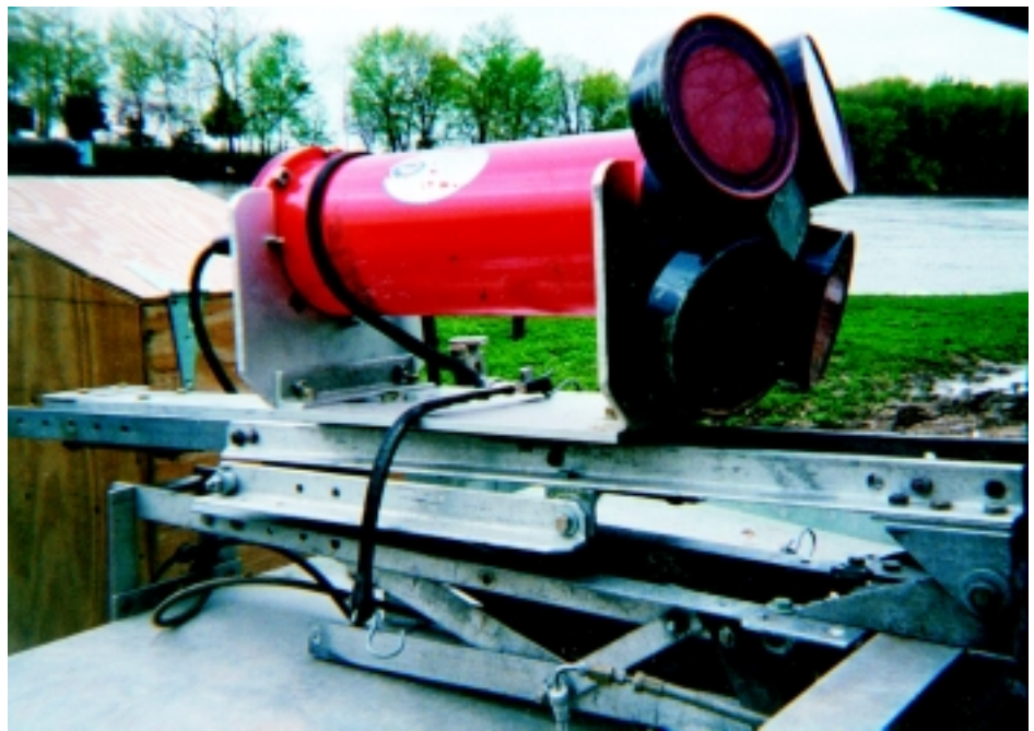
Figure 8. An acoustic doppler current profiler (ADCP) is used to find the discharge of a stream by using sound waves to determine the area and velocity of the water.
