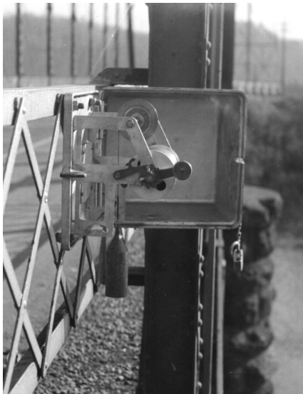
Figure 3. A wire-weight gage used to measure stage (or depth), mounted on the side of a bridge.
