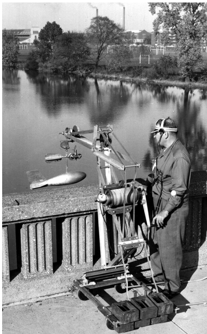
Figure 1. Stream gager making a streamflow measurement using a bridge crane and a current meter. Picture taken in the 1940's from a bridge near The Ohio State University (OSU). OSU worked with the USGS to build a stream-gaging-station network in Ohio.
