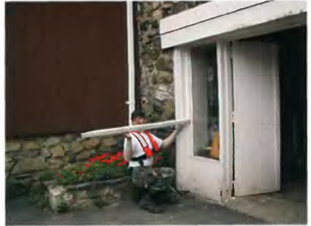
Figure 3. Photograph of high-water mark on the Culligan Building near the Station Road bridge upstream from Glen Brook in Sparta Township, N.J.
