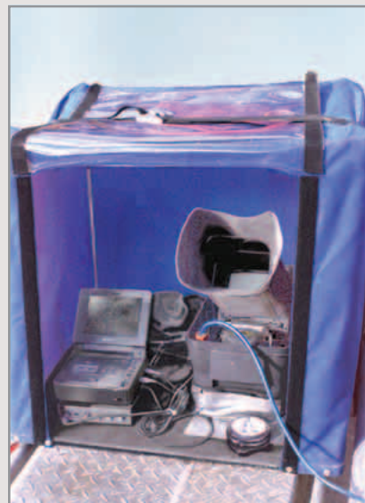
Topside video console, including video monitor and digital recorder
