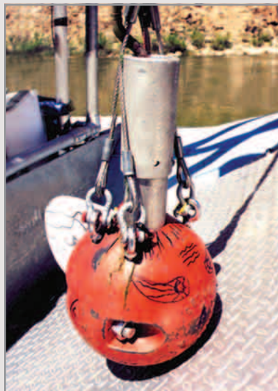
Video camera assembly including stabilizer fin, camera pressure case, and bridle assembly.
