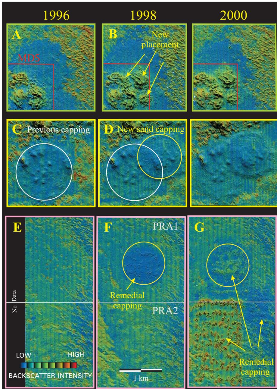
Figure 6. Pseudo-colored backscatter intensity and shaded relief map of parts of the HARS in 1996, 1998, and 2000 (see fig. 4 for location). These images illustrate changes in the sea floor topography and backscatter intensity that occurred between 1996 and 1998 and between 1998 and 2000 caused by placement of dredged material and by remedial capping. See text for a description of these images and major features.
