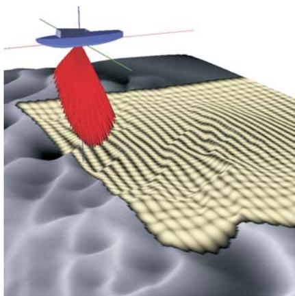
**Figure 3.** High-resolution multibeam mapping systems use sound from an array of transducers to measure water depth and sediment characteristics of the sea floor. The horizontal resolution of the maps is a few meters, providing an image of the sea floor topography and sediment properties somewhat comparable to an aerial photograph.
