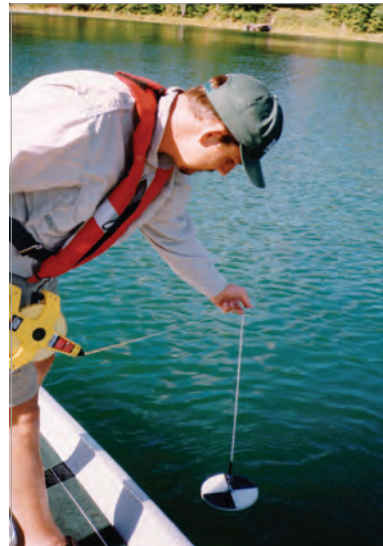
USGS scientist measuring the transparency of water using a Secchi disk. Photo by Russ Minnerick.
