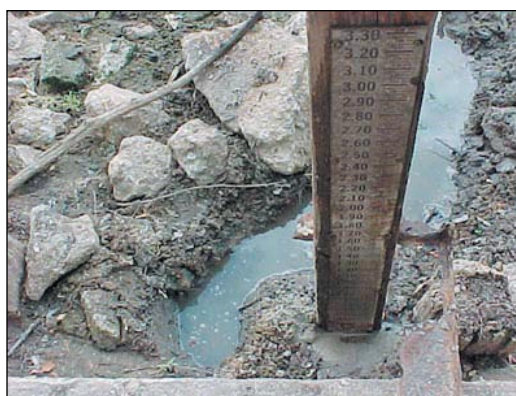
USGS streamflow monitoring station on the Ogeechee River, Georgia, during July 2000. Low streamflow during drought periods affects the quantity and quality of streamwater and reduces the assimilative capacity of the stream to handle waste discharges. Data from the USGS streamflow monitoring network for Georgia provides real-time information on streamflow during drought periods to enable water-resource managers to make informed decisions regarding water withdrawal and waste discharges.
