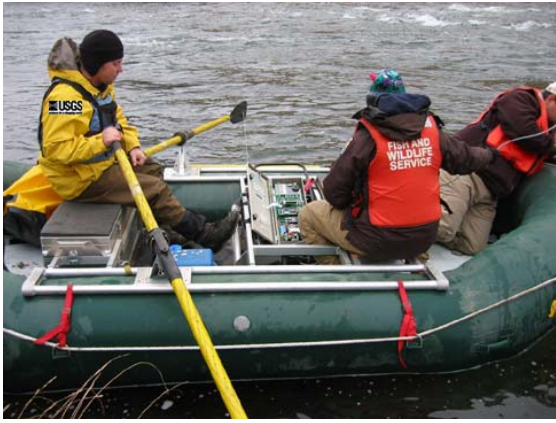
USGS and U.S. Fish and Wildlife Service biologists experiment with a detection system for locating tagged juvenile Chinook salmon.
