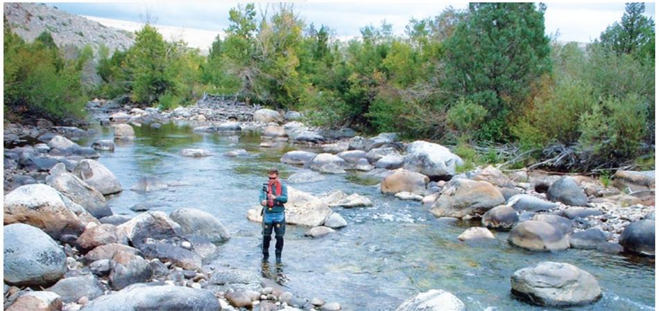
**Discharge measurement during drought conditions.** A USGS streamgager measures discharge at North Fork Little Wind River near Fort Washakie, Wyoming, August 28, 2002. Photo by Jerrod Wheeler, U.S. Geological Survey.
