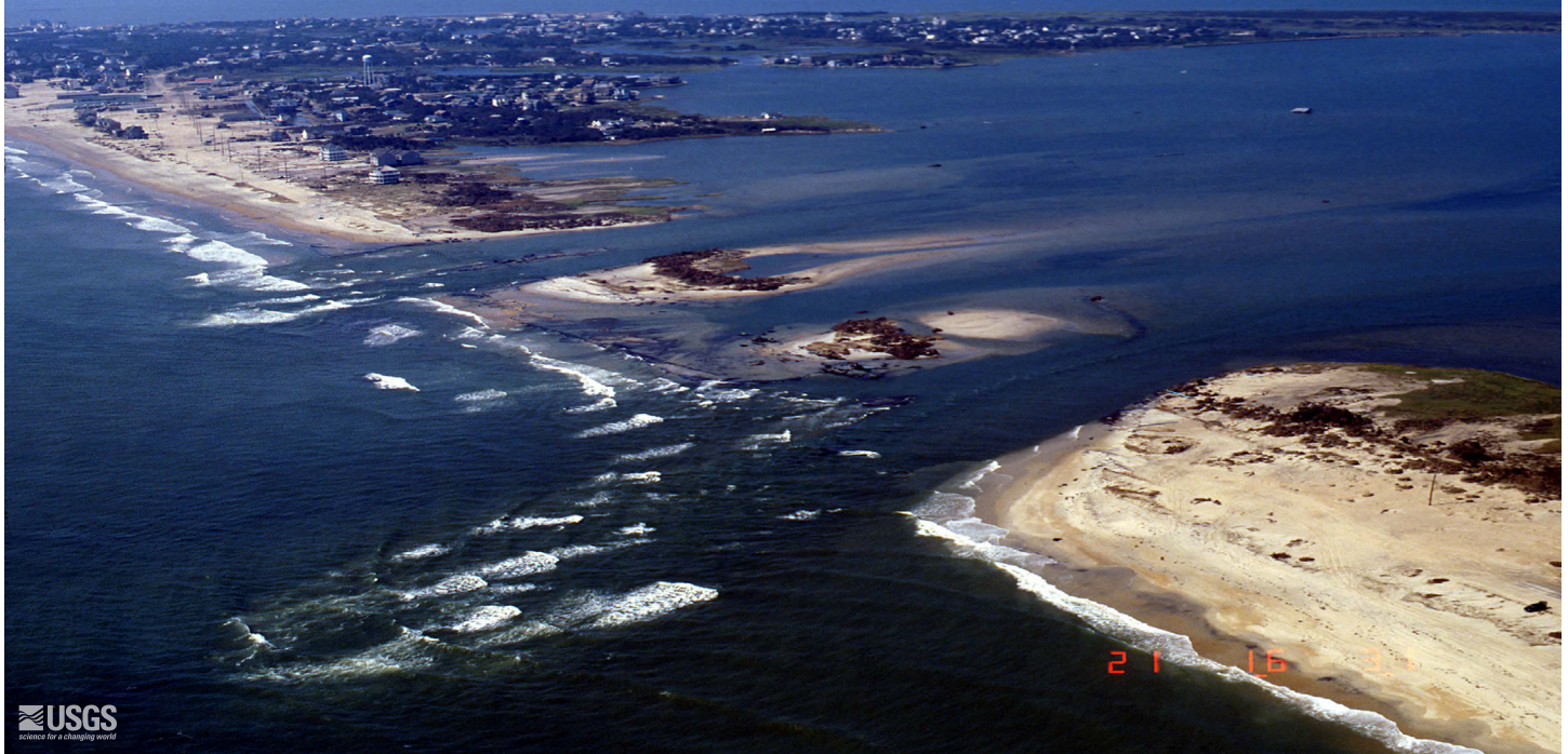
Figure 2. Hurricane Isabel opened a breach in the island southwest of Cape Hatteras. Combined waves and storm surge attacked the island where the dunes were lowest and the island was narrowest.
