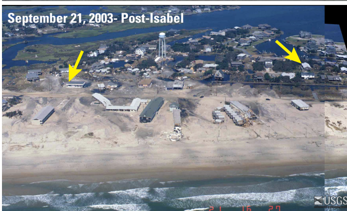
Figure 4. Hatteras Village, North Carolina. USGS aerial photography taken before and after the landfall of Hurricane Isabel. Storm surge and waves destroyed and inundated the dunes protecting the hotels. The water washed the buildings from their foundations and covered roads with sand. (Arrows in all images point to the same features.)
