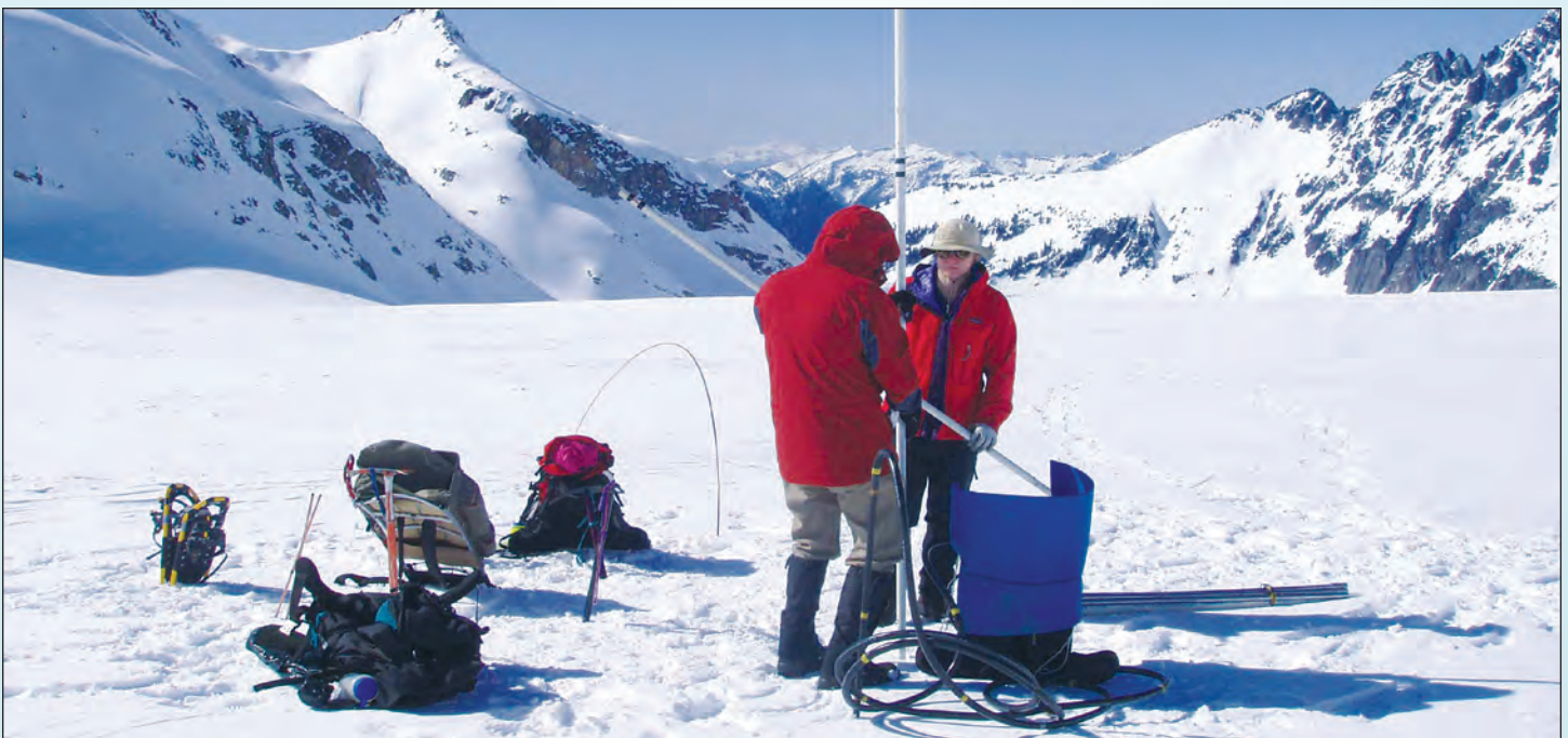
Figure 4. Setting a measurement stake at South Cascade Glacier, Washington.
