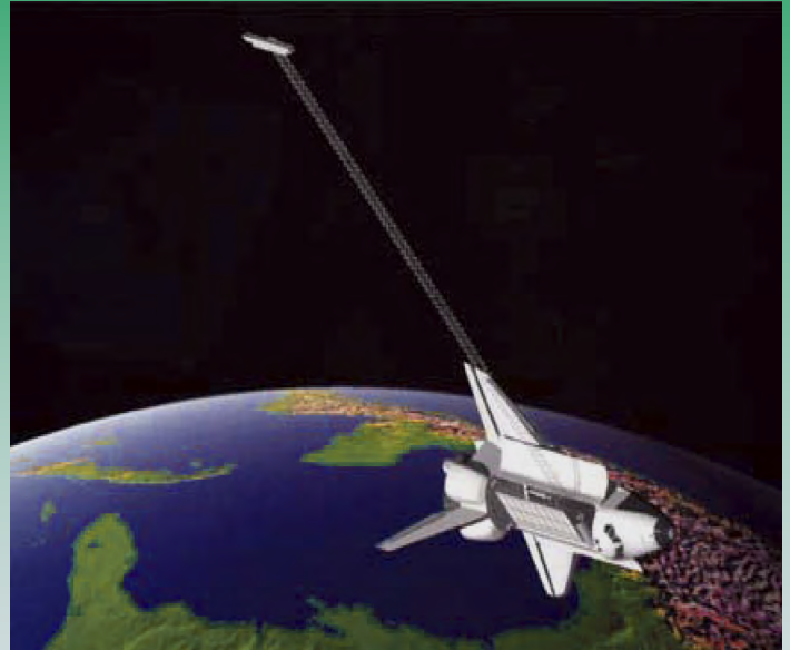
Artist's rendering of Space shuttle Endeavour and the 200-foot long SRTM antenna deployed for image acquisition.
