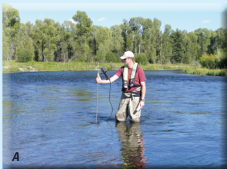
(A) Making a summer streamflow measurement at site A-R7; (B) evaluating aquatic plants; (C) collecting algal samples; and (D) making a fall streamflow measurement at site A-R6D. (Photographs by Cheryl A. Eddy-Miller [A] and Jerrod D. Wheeler [B, C, and D].)
