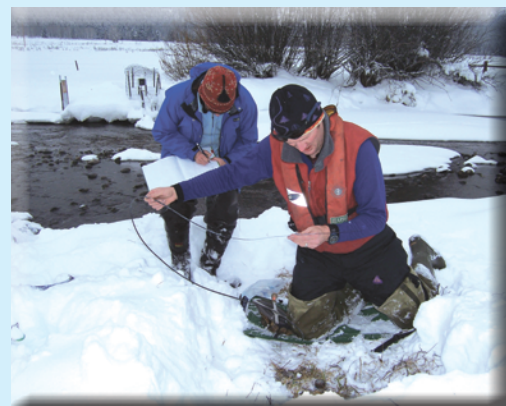
Measuring water levels at well cross section. (Photograph by Rodney R. Caldwell.)
