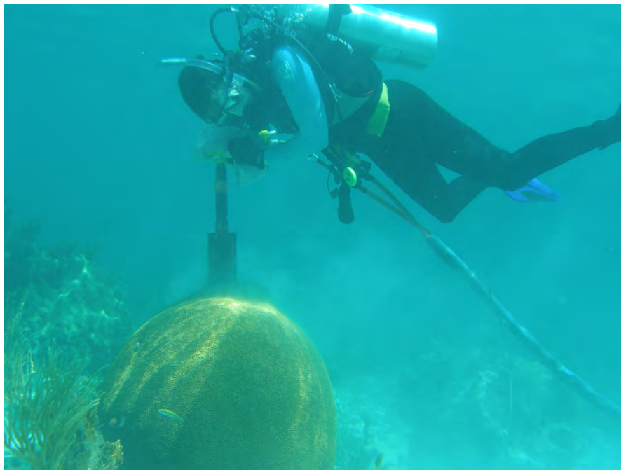
Figure 2. A USGS researcher takes a core of the coral species Diploria strigosa . A core barrel is used with a rotary coring device to obtain 4-inch-diameter cylinders of coral skeleton, typically of several feet in length. Photo credit: Kristine L. DeLong, Louisiana State University.
