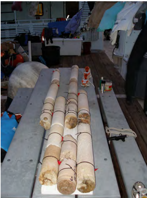
Figure 3. Cores drilled from corals are drying on the table. Samples from the coral cores are analyzed to provide information on coral growth rates and variations in ocean temperature and salinity over time. Photo credit: Christopher D. Reich, USGS.
