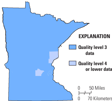
Figure 1. Map of Minnesota showing the areal extent and quality levels of planned and existing publicly available light detection and ranging (lidar) data in November 2012. No lidar data that meet 3DEP requirements for quality level 2 or better are publicly available for Minnesota. See table 2 for quality levels.
