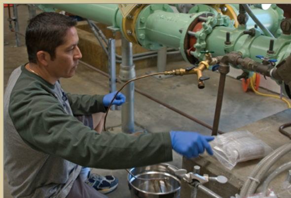
Sampling a public-supply well in San Bruno, CA. Photograph by Cathy Munday, U.S. Geological Survey
