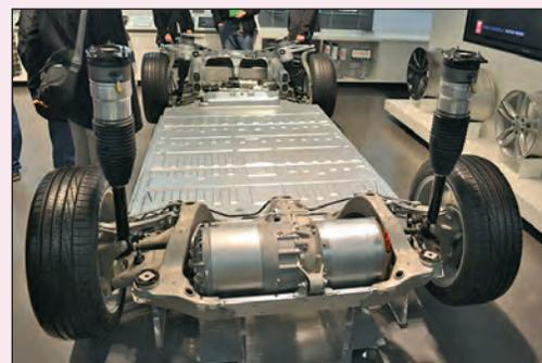
View into a Tesla Model S® electric car showing the lithium-ion battery covering most of the bottom of the chassis. Various battery configurations use between about 10 and 22 kilograms of lithium. Photo by Oleg Alexandrov, downloaded from Wikimedia Commons.
