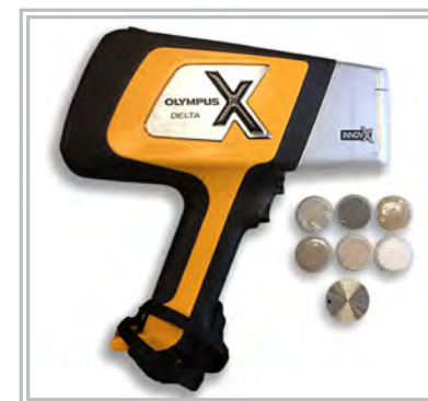
Figure 2. Handheld X-ray fluorescence spectrometer and external calibration standards.
