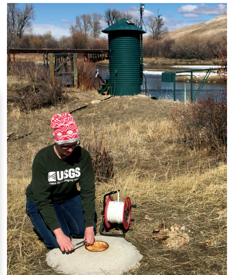
Figure 6. U.S. Geological Survey scientist accesses a well on the west side of the New Fork River near Big Piney, Wyoming. Instrumentation in the well and in the river continuously measure water levels and temperature and transmit the data to the nearby streamgage (green structure in the background). By comparing well and streamgage data, scientists determined that some water flows from the river into the groundwater in summer months, whereas in the winter months water flows from groundwater into the river.
