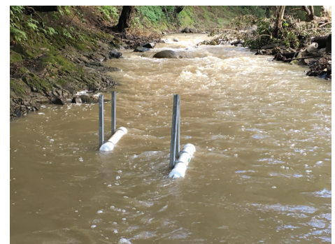
Figure 2. Example of passive samplers used to collect suspended-sediment samples for target sediment. Prior to planning for the target sediment sampling design, it is important to contact the laboratory where the analyses of the various properties selected for the study will be performed to ask questions pertaining to sample mass and holding requirements; for example, whether the samples should be refrigerated. [Photo of Crow Creek, California by Allen Gellis, USGS, January 31, 2017]
