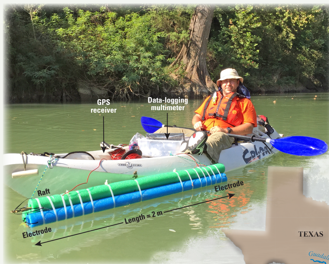
Figure 1. Geophysical measurement equipment and typical streamflow conditions in the Guadalupe River, south-central Texas, during the self-potential survey, September 2016. [GPS, Global Positioning System; m, meter. Photograph by C. Hartman, U.S. Geological Survey]
