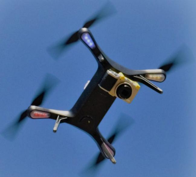
A Pentax Ricoh GR11 natural-color, high-resolution, global shutter digital camera mounted on the bottom of a 3DR Solo quadcopter drone; by Sandra Brosnahan, U.S. Geological Survey. This configuration is used to take aerial photographs for photogrammetric mapping.
