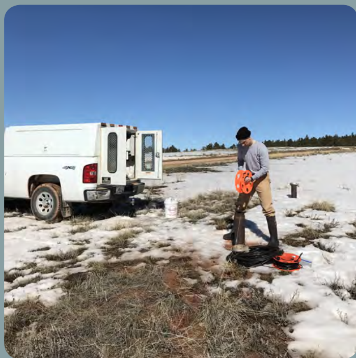
Figure 8. U.S. Geological Survey hydrologist measuring the depth to water in a well near Jewel Cave National Monument.
