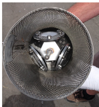
Figure 2. Deployment canister containing three polar organic integrative samplers mounted on a center bracket.
