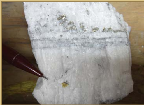
Visible gold, telluride, and sulfide minerals in quartz from Kensington Mine. Photograph by S. Karl, U.S. Geological Survey.
