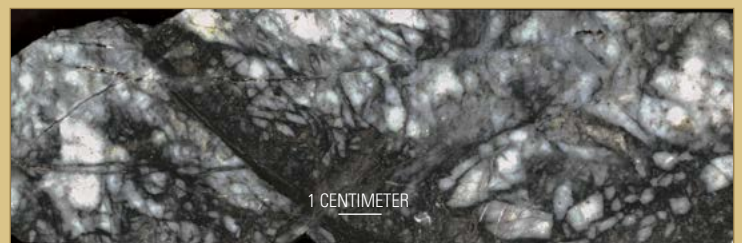
Sulfide vein in altered diorite from the Jualin Mine (top). Photograph by S. Karl, U.S. Geological Survey. Brecciated gold-bearing quartz-arsenopyrite vein from the Pogo Mine in eastern interior Alaska (bottom), photograph used with permission.
