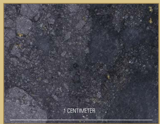
Brecciated gold-bearing quartz-arsenopyrite vein from the Pogo Mine in eastern interior Alaska, photograph used with permission.
