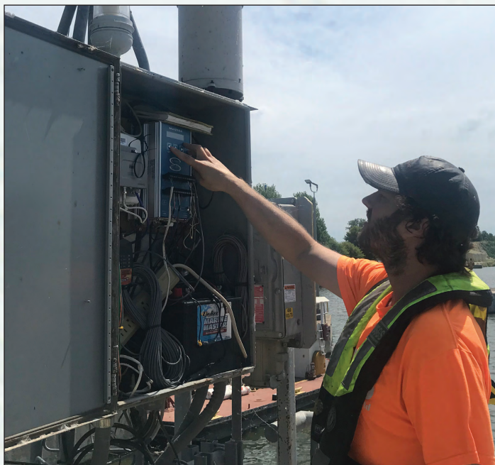
U.S. Geological Survey scientist checking a streamgage at Starved Rock Lock and Dam, Ottawa, Illinois. Photograph by the U.S. Geological Survey.
