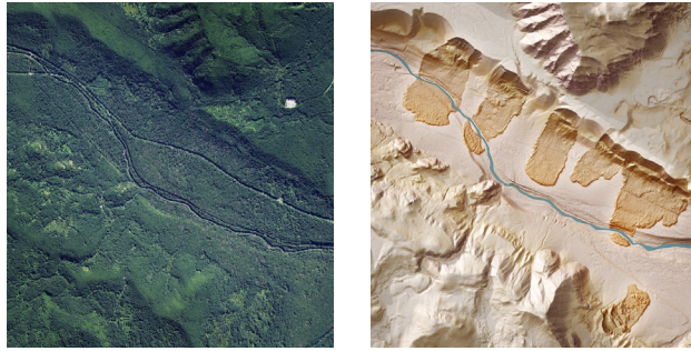
Figure 2. Comparison of aerial photograph (left) and lidar-derived image (right) of the Cedar River, King County, Washington. Landslide activity is not readily apparent in the former but is visible in the latter. At least six landslides can be seen in the lidar-derived image. Graphics courtesy of the Washington Geological Survey.
