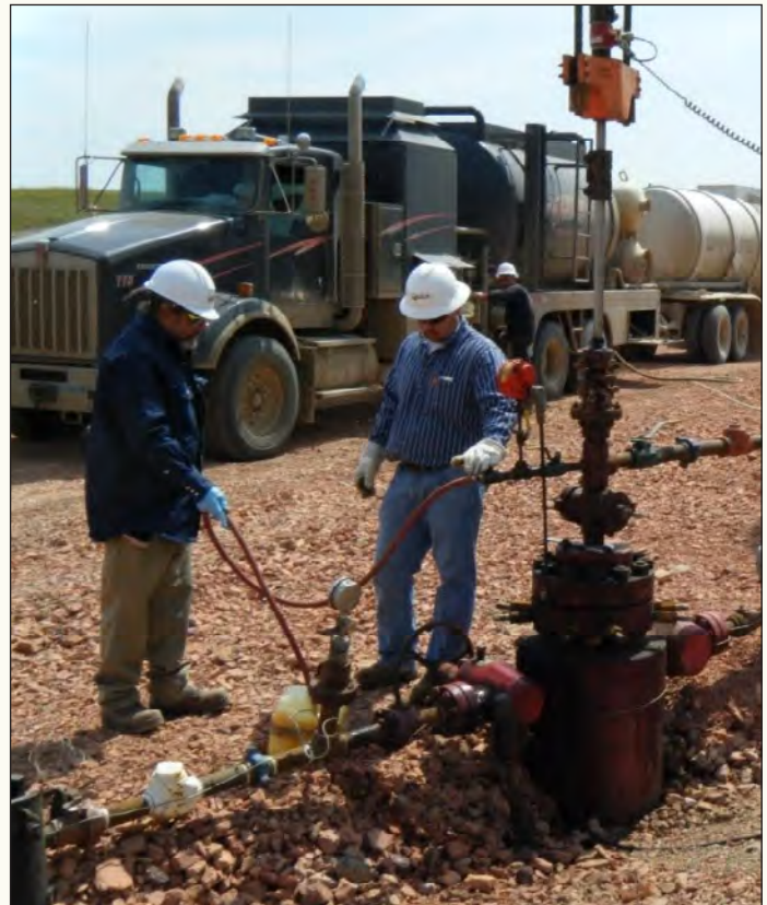
Figure 4. Collection of a produced-water sample. A truck injecting fresh water into an oil well for routine maintenance is shown in the background (photograph by Joanna Thamke, U.S. Geological Survey).
