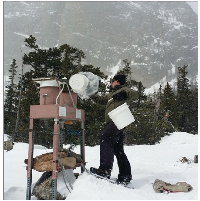
Swapping a clean precipitation collector with a collector from the previous week at Loch Vale in Rocky Mountain National Park.
