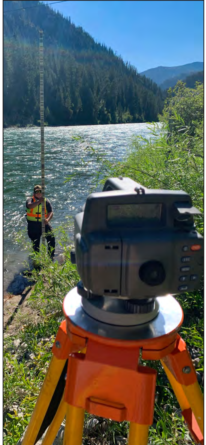
U.S. Geological Survey employee surveys streamgage datum for the Snake River near Alpine, Wyoming. Photograph by Cheryl Eddy-Miller, U.S. Geological Survey.
