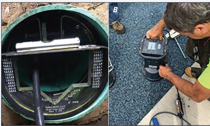
Figure 4. Runoff instruments installed at Virgil I. Grissom Fine and Performing Arts Elementary School. A, a six-inch V-notch weir installed with, B, a sewer flow meter in a sewer line draining the green infrastructure. Photographs by Clint Bailey, U.S. Geological Survey.
