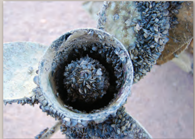
Invasive mussels encrust a propeller, making it inoperable (photograph by the National Park Service).
