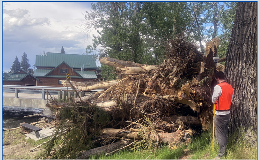
U.S. Geological Survey staff surveying a high-water mark (debris line) along Rock Creek in Red Lodge, Montana. Photograph taken by Seth Siefken, U.S. Geological Survey, on June 29, 2022.
