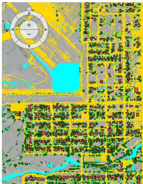
Figure 2. Perspective view of a part of Roswell, New Mexico, derived from lidar point-cloud data. Image shows bare-earth ground in gray, vegetation canopy in green, building footprints in red, impervious surfaces in yellow, and potential flood-prone depressions in blue. Graphic courtesy of Earth Data Analysis Center, University of New Mexico.
