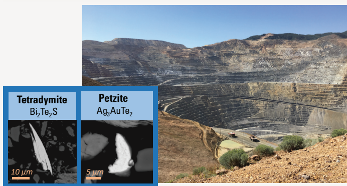
Figure 2. Tellurium is hosted in a variety of minerals in tailings (left) generated by the Bingham Canyon mine in Utah (right), which recovers copper, molybdenum, and gold and byproducts including tellurium. Photograph by Bob Seal, U.S. Geological Survey.
