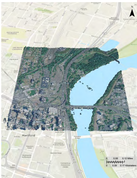
Figure 2. A sample of 3DEP lidar point cloud quality level 2 data as downloaded from The National Map (TNM), colored by imagery from the National Agriculture Imagery Program Plus (1 meter to 1 foot), also downloaded from TNM. The sample displayed is located in Hartford, Conn., where the Connecticut River flows under the Interstate 84 (U.S. Route 6) bridge.
