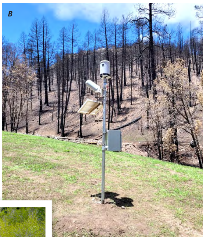
Figure 5. A, U.S. Geological Survey staff downloading data from 401723105400101 Andrews Creek Meteorological Station at Rocky Mountain National Park, Colorado. B, U.S. Geological Survey precipitation gage deployed in a wildfire burn scar to be used for flood warning. Photographs by U.S. Geological Survey.
