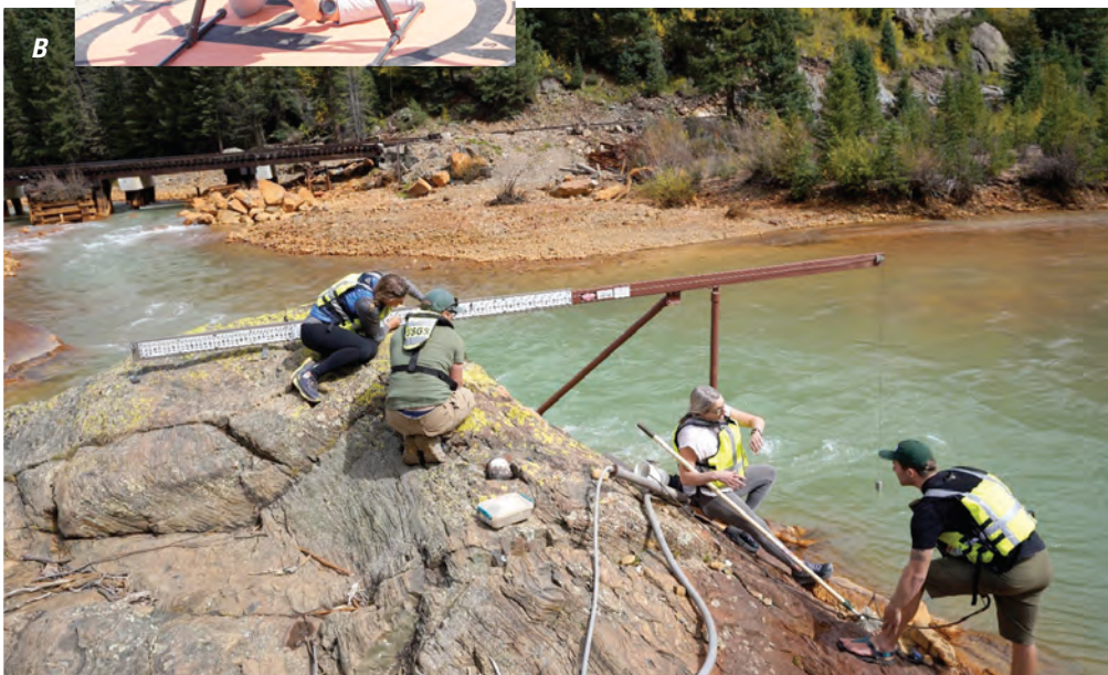
Figure 7. A, U.S. Geological Survey staff programming data collection sensors on an uncrewed aircraft system. B, U.S. Geological Survey staff servicing water quality data collection sensors at the streamgage 09359020 Animas River Below Silverton, Colorado. Photographs by U.S. Geological Survey.
