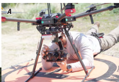
Figure 7. A, U.S. Geological Survey staff programming data collection sensors on an uncrewed aircraft system. B, U.S. Geological Survey staff servicing water quality data collection sensors at the streamgage 09359020 Animas River Below Silverton, Colorado. Photographs by U.S. Geological Survey.
