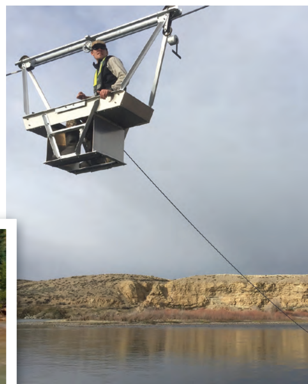
Figure 8. U.S. Geological Survey staff making an acoustic Doppler current profiler measurement from a cableway at U.S. Geological Survey 09211200 Green River below Fontenelle Reservoir, Wyoming streamgage. Photograph by U.S. Geological Survey.
