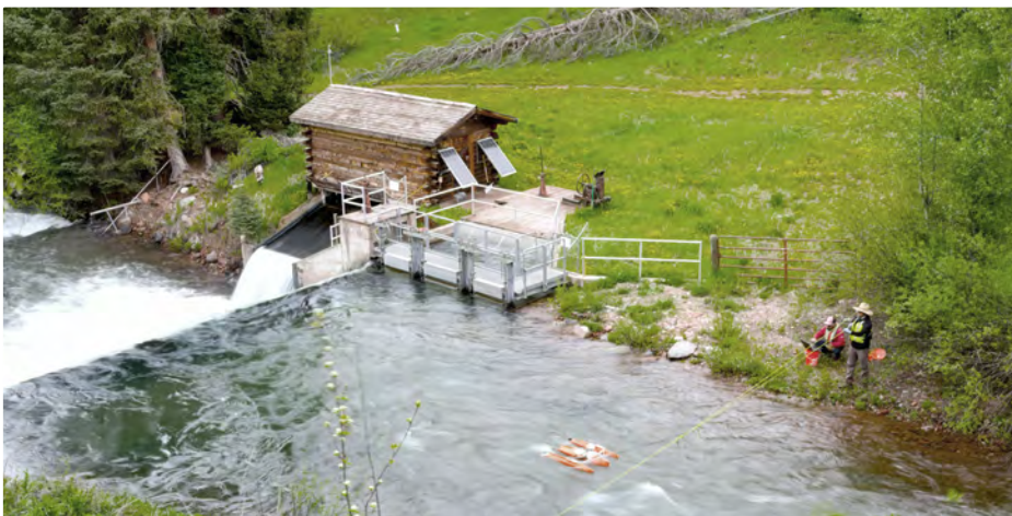
Figure 3. U.S. Geological Survey staff making a streamflow measurement using an acoustic Doppler current profiler at U.S. Geological Survey 09076000 Maroon Creek near Aspen, Colorado streamgauge. Photograph by U.S. Geological Survey.
